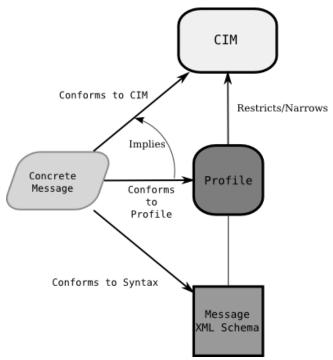
Figure 2, Concrete Message Generation
