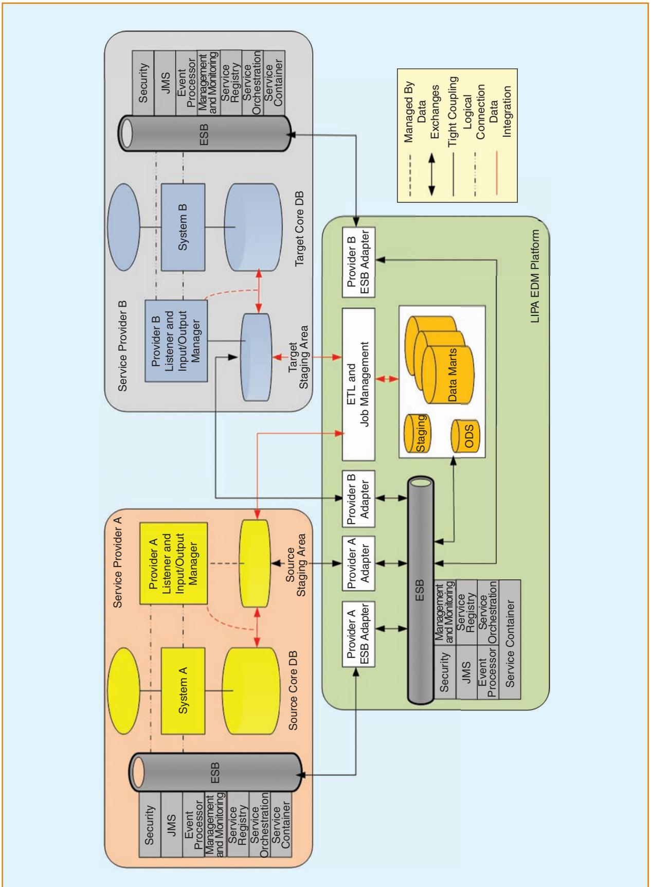
**figure 5.** Patterns for service provider data integration.
